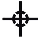
Fig. 1: Symbol for marking the center of gravity
