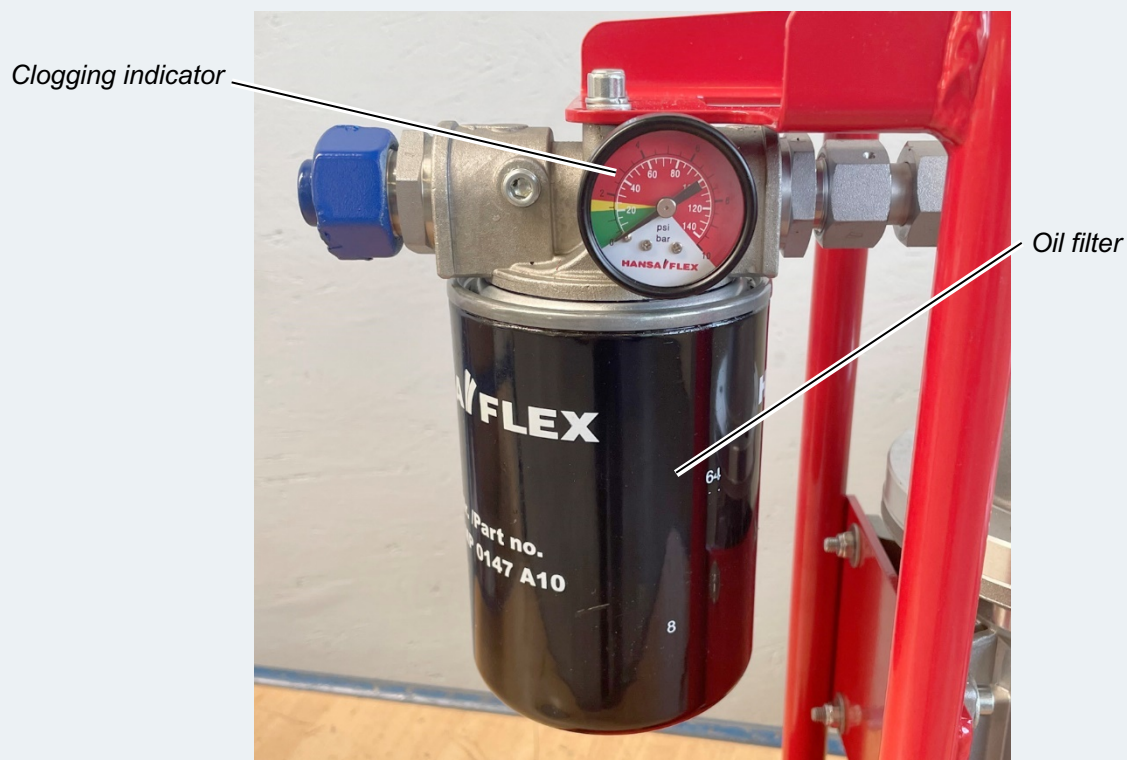
Figure 5: Oil filter with clogging indicator
